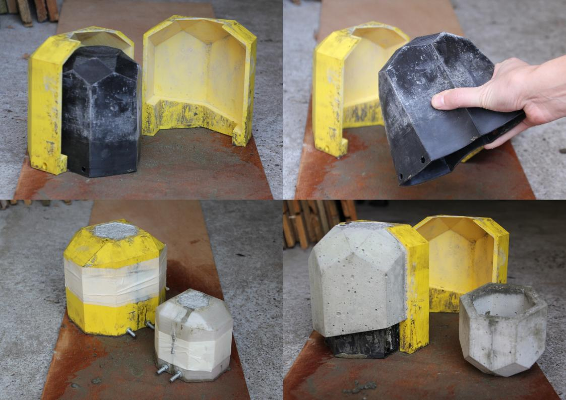
The concrete planters are made using 3D printed moulds. Two halves form the outside mould, these are made of PLA, which is a very stiff material, the most commonly used material for 3D printing.
